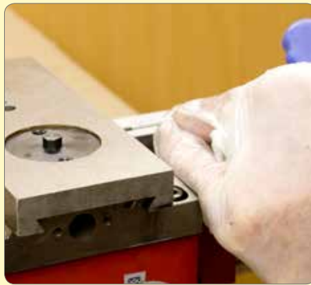
149. Fit adjusting screws and adjust so slide can be moved back and forth easily by hand.
