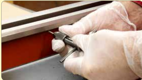
86. Drill and tap the fixing holes deeper if necessary.
