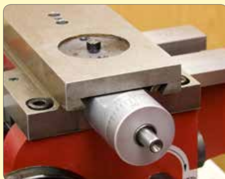
160. Remove the handle again in order to fit the micrometer dial and friction spring.
