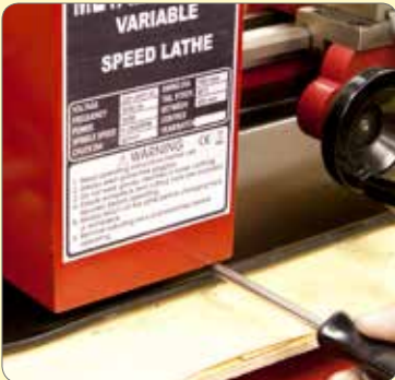
36. Remove 4 screws retaining the control panel and lay it down beside the machine.
