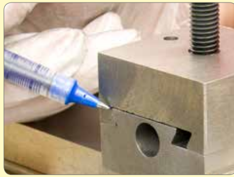
163. Temporarily fit top slide to compound base and check for clearance in corners of dovetail.
