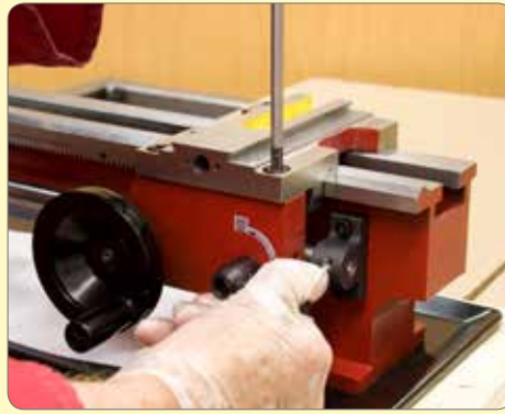
108. Lock 1/2 nut onto leadscrew and tighten apron fixing screws.
