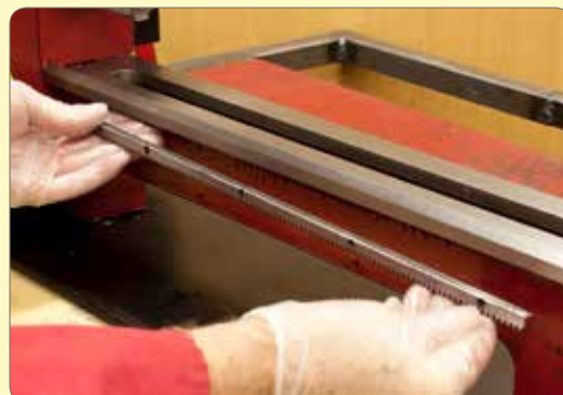
32. Remove the rack from the front of the bed.
