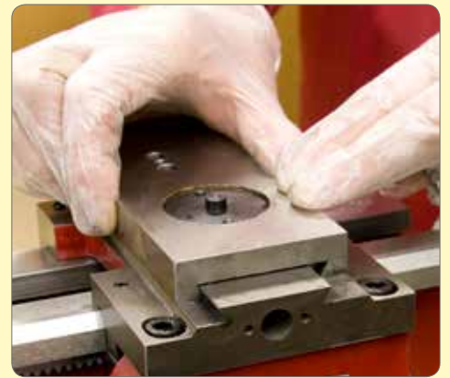
149. Fit adjusting screws and adjust so slide can be moved back and forth easily by hand.
