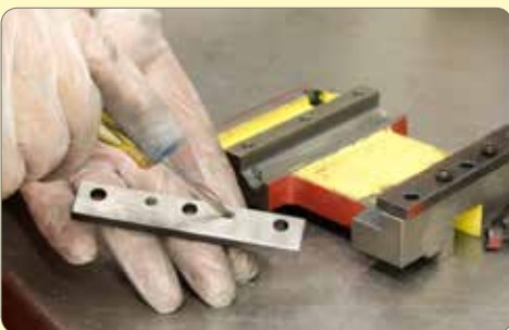
91. Loosen shear plate adjusting screws below the level of the plate and loosely fit to saddle.
