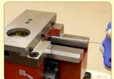
144. Fit adjusting screws lightly.
