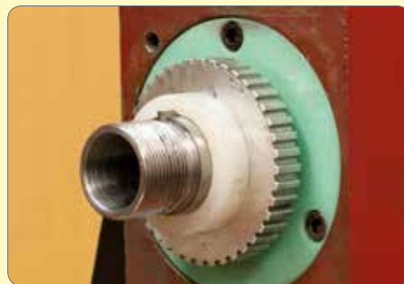
61. Fit the key and plastic spacer.
