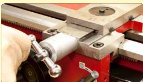
20. Wind the cross slide off the feed screw.
