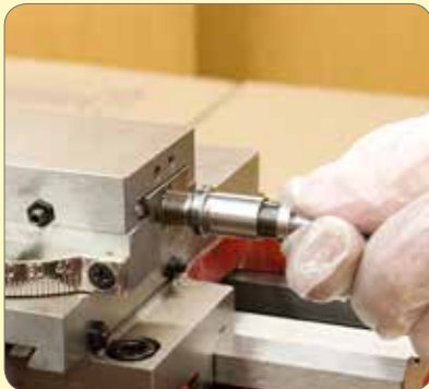
167. Oil / grease feed screw and fit. Oil / grease end of feed screw and bracket and fit.
