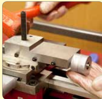
15. Tap the compound slide to remove the micrometer dial taking care not to lose the friction spring.
