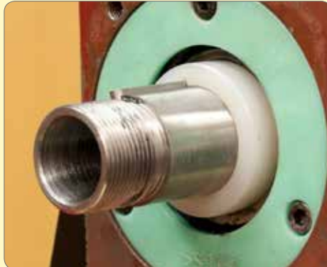
61. Fit the key and plastic spacer.
