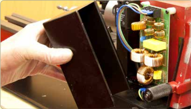
34. Remove the power board cover.
