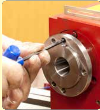
45. Remove the front bearing cover screws.
