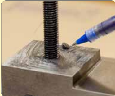
174. Grease and fit the tool post spring and plunger and fit the tool post.
