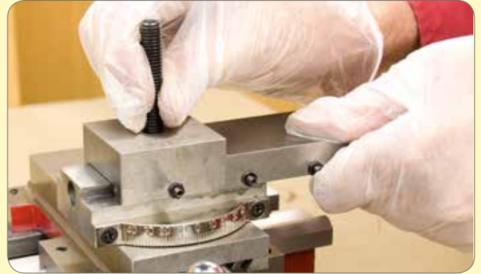
166. Adjust the screws so the slide will move back and forth easily by hand.
