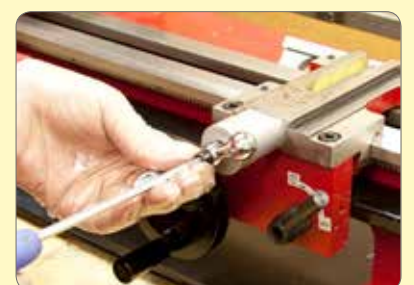
22. Remove the ball handle & washer.
