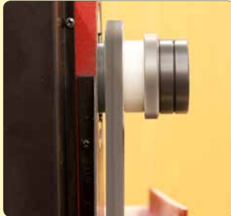
80. Run the spindle following the procedure below and check the belt is centred on the pulley. If not the motor angle may be adjusted by slackening these screws. Check the belt tension again.
