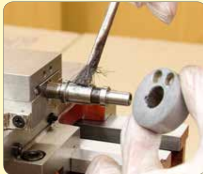
167. Oil / grease feed screw and fit. Oil / grease end of feed screw and bracket and fit.
