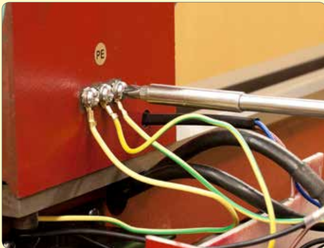
71. Reconnect the earth wires to the head.
