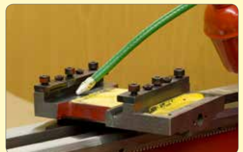
92. Oil bed and saddle and slide saddle onto bed.
