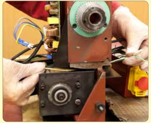
67. Thread wires from bottom of motor board through motor cover and then through bed to front.
