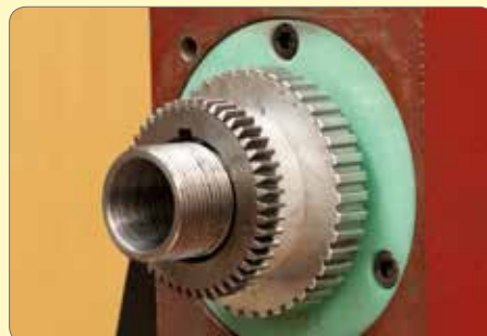
64. Fit the outer spacer and gear.
