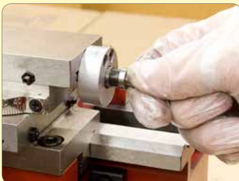
168. Turn the feed screw to check it turns freely.
