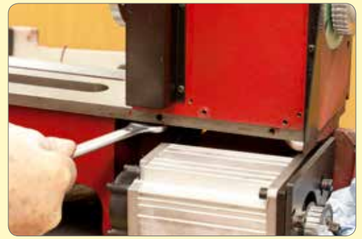
43. Remove the 2 hex socket and 2 hex head screws securing the head to the lathe bed.
