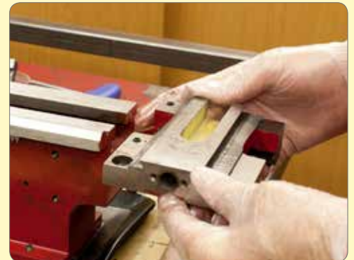
30. Slide the saddle off the end of the bed.
