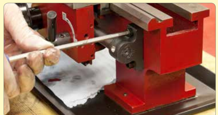
105. Grease end of leadscrew and feed through 1/2 nut and into bracket at headstock end.
