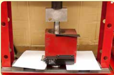
48. Press out the spindle assembly.
