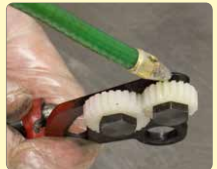
116. Oil the tumbler reverse gear shafts.
