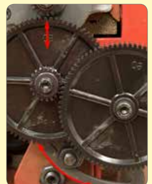
129. Engage quadrant and adjust backlash between gears A and B.
