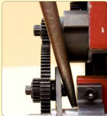
126. "Tweak" the lower quadrant bracket until the gears are in proper alignment.
