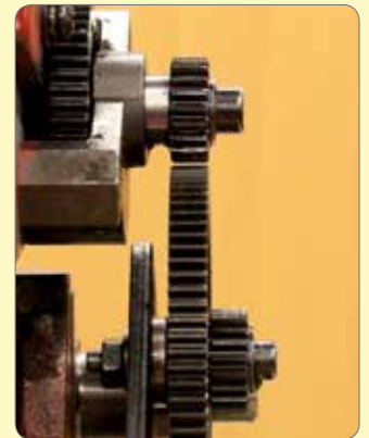
124. Temporarily fit the gear quadrant. DO NOT engage the gears.
