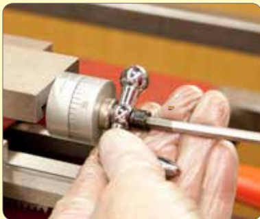
14. Remove the ball handle and spacer.
