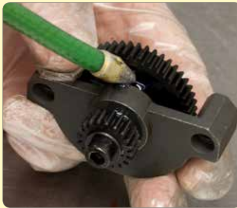
120. Oil the transfer gear shaft.
