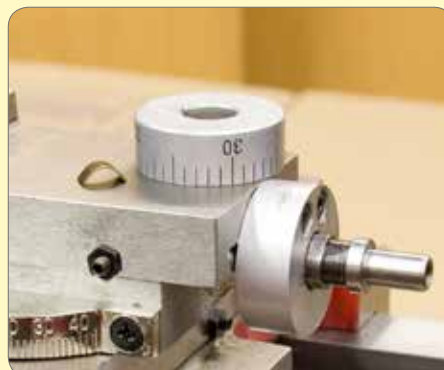
169. Assemble and fit the micrometer dial and friction clip to feed screw.
