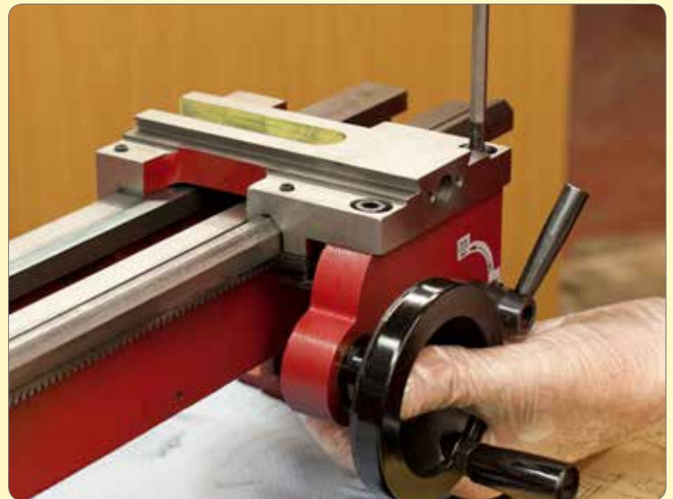
99. Oil and/or grease the gears and shafts, dovetail and half nut of the apron assembly. Check 1/2 nut dovetail is correctly adjusted by operating the lever.
