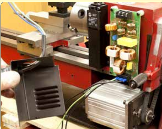
40. Remove motor end cover and mains cable
