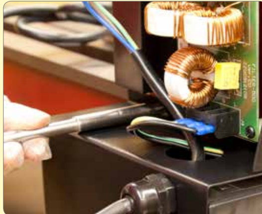
39. Remove the motor cover and pull power cables through from front of machine.
