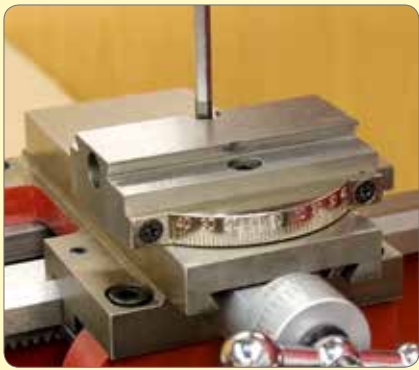
162. Fit compound base to cross slide.
