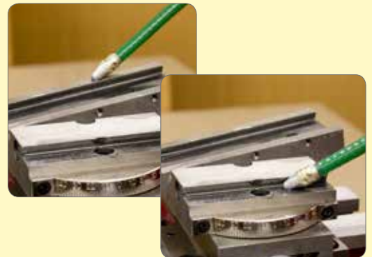
164. Oil top slide assembly and fit.
