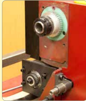
9. Remove the tumbler reverse lever assembly.
