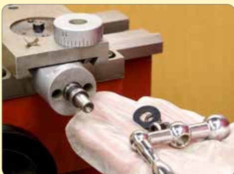
160. Remove the handle again in order to fit the micrometer dial and friction spring.
