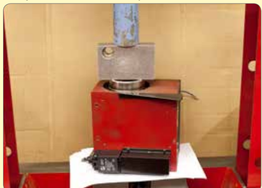
54. Press front and rear outer bearing races into the head.
