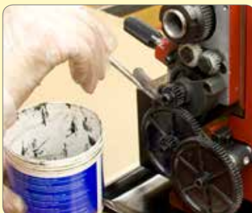
130. Very lightly grease gears.
