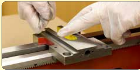
86. Drill and tap the fixing holes deeper if necessary.
