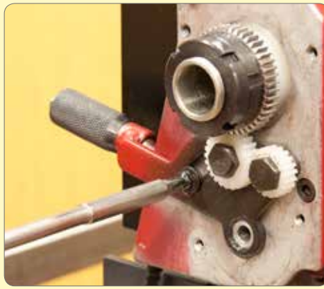
9. Remove the tumbler reverse lever assembly.
