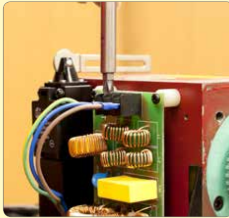
69. Connect Mains In to top of board.
