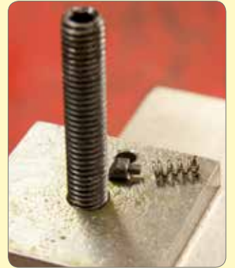
13. Remove the detent plunger & spring from the compound slide.
