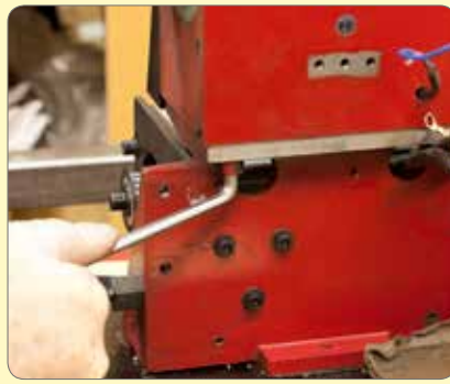
43. Remove the 2 hex socket and 2 hex head screws securing the head to the lathe bed.
