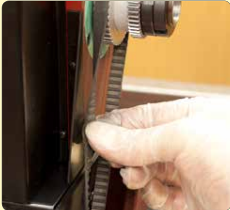
79. When adjusting belt tension, it should twist easily through 90°
