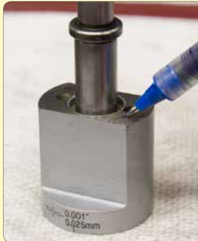
140. To increase backlash, machine a little from the recess. Remove the feed screw and bracket and put to one side.
