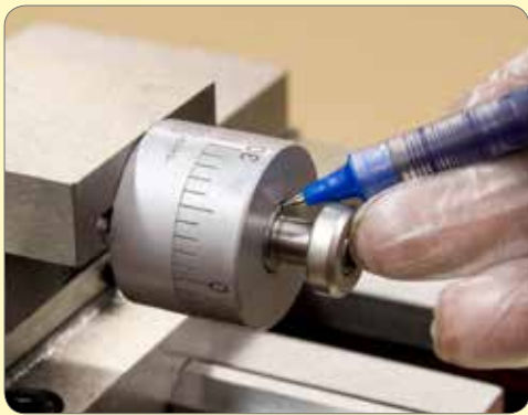
172. Backlash can often be reduced by turning a recess in the spacer to clear the shoulder on the end of the feed screw. The recess depth should be slightly less than the measurement taken with the feeler gauge to allow some clearance. Adjust for free movement with minimal backlash.
