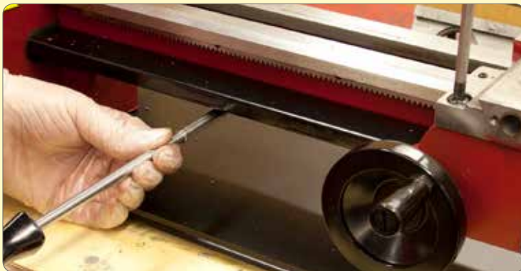
28. Undo the screws retaining the lead screw cover...
