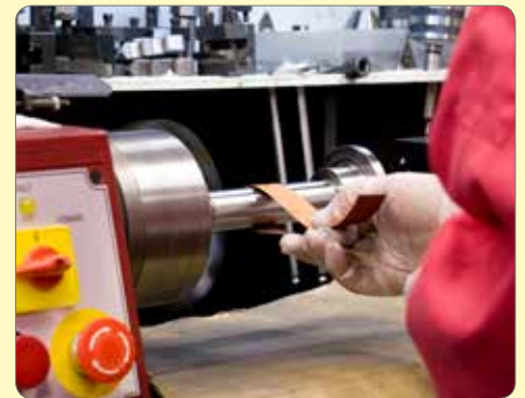
52. Polish the spindle and test the fit by using one of the old bearings (if not damaged).
