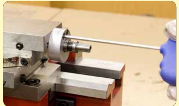
166. Adjust the screws so the slide will move back and forth easily by hand.
