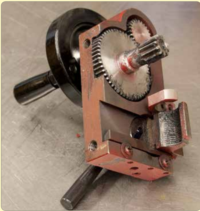
99. Oil and/or grease the gears and shafts, dovetail and half nut of the apron assembly. Check 1/2 nut dovetail is correctly adjusted by operating the lever.
