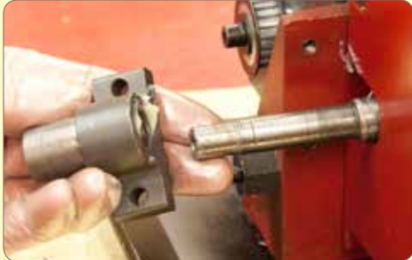
26. Remove left hand and right hand lead screw carrier brackets.
