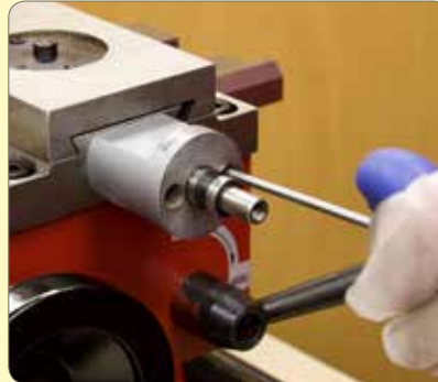
151. Assemble onto the saddle.
