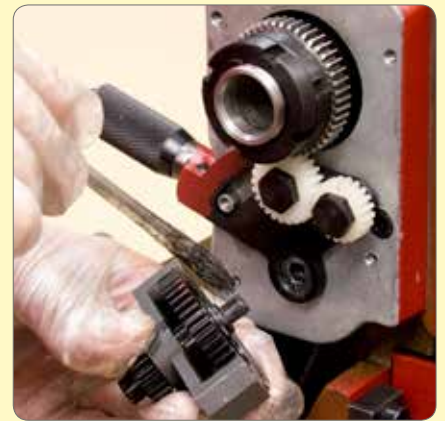
121. Grease the transfer gear shaft.
