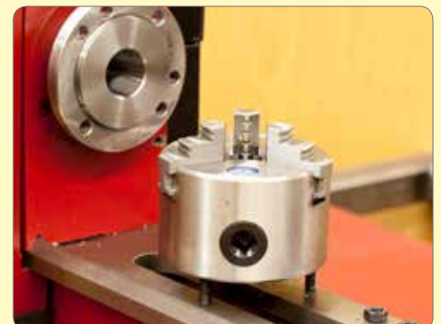
33. Remove the chuck from the spindle flange.
