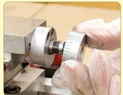
169. Assemble and fit the micrometer dial and friction clip to feed screw.
