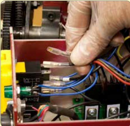
38. Disconnect power cables and guard switch wires.
