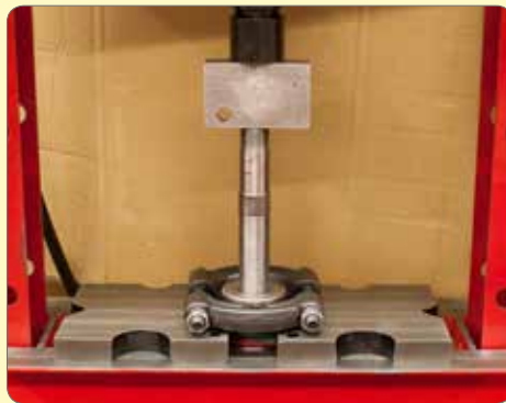
49. Press out the rear bearing.
