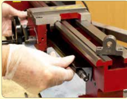
134. Remove right hand leadscrew bracket and fit screw guard.
