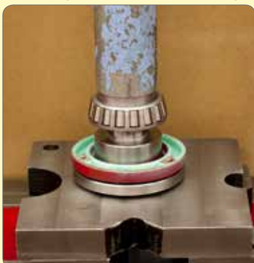
53. Fit bearing cover and press on nose bearing.
