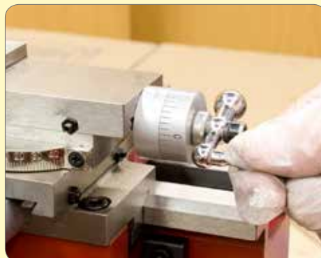
169. Assemble and fit the micrometer dial and friction clip to feed screw.
