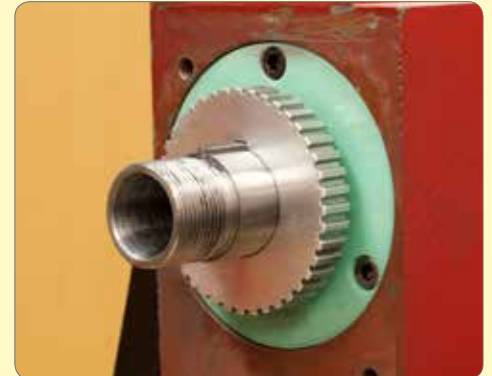
62. Fit the spindle drive belt pulley.
