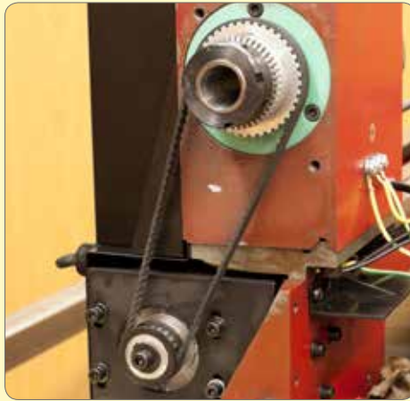
77. Fit the drive belt and adjust the belt tension.
