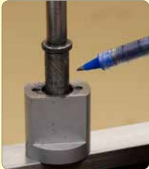
150. Grease / oil the feed screw and bracket.
