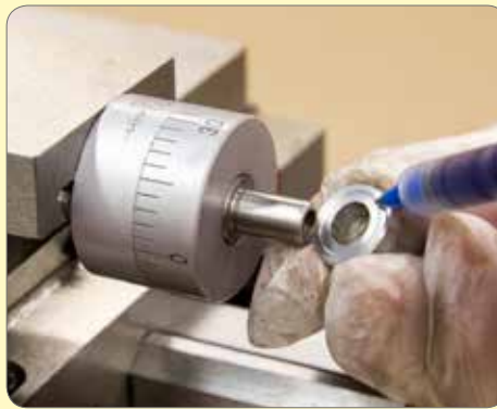
172. Backlash can often be reduced by turning a recess in the spacer to clear the shoulder on the end of the feed screw. The recess depth should be slightly less than the measurement taken with the feeler gauge to allow some clearance. Adjust for free movement with minimal backlash.
